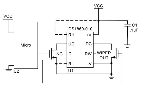
The timing requirements for the pulses are the same as with the pushbutton setup. But by using the microprocessor, the UC and DC inputs can be quickly pulsed to reach either limit and thus a known position. The microprocessor can then pulse the inputs pins to place the wiper at a desired position.
