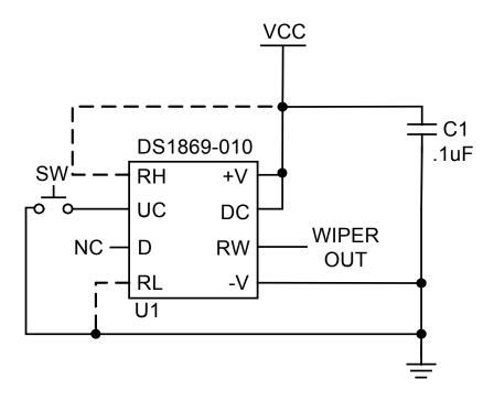
SINGLE CONTACT MODE USING A MICROPROCESSOR SIGNAL Figure 4
